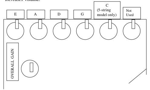
Diagram - Internal Preamp and Trim Pot Controls
