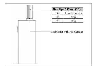
1.5 Connect a flue pipe by inserting it into the flue spigot and sealing using fire cement.
