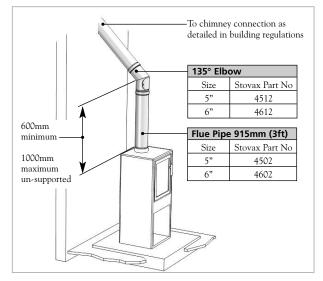
1.7 As it is not possible to fully sweep the flue through the stove, provision must be made to clean the flue and collect debris without removing the stove.
