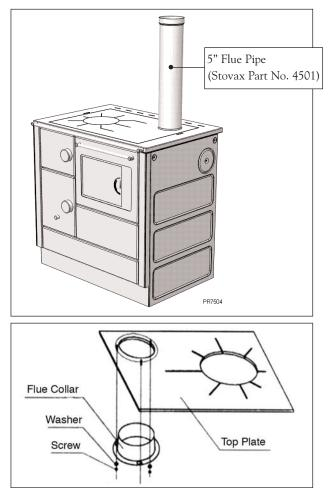
1.15 Connect a flue pipe 612mm long (Stovax part no 4501 (5" pipe)) by inserting it into the flue spigot and sealing using fire cement.
