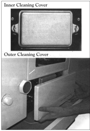
After removing the outer cover by pulling free from the sprung retaining clips the inner cover can be removed after unscrewing the two, wingnut fixings. Care should be taken not to damage any seals. If seals are damaged they should be replaced before cooker is re-used.
