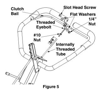
**NOTE:** Do not overtighten clutch cable. Too much tension may cause it to break.
