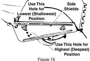
When breaking up sod and for shallow cultivation, use the setting which gives 1" of tilling depth (second hole from the top). Place the side shields in their lowest position. For further depth, raise the depth stake and side shields and make one or two more passes over the area.
