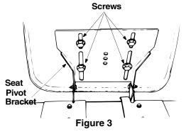
**NOTE:** The seat may have been shipped in a box. Remove the four screws from the bottom of seat and place seat in position against the seat pivot bracket. Follow the directions above to attach the seat.
