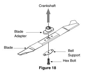
• Install the blade adapter on the crankshaft with the "star" away from the engine. Place the blade with the side marked bottom (or with part number) facing away from the adapter. Align the blade bell support over the blade with the tabs in the holes of the blade and insert the hex bolt. Tighten the hex bolt to the torgue listed here.
