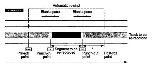
Post-roll is 10 counts on the tape counter at 9.5 cm/sec (5 counts at 4.8 cm/sec).
