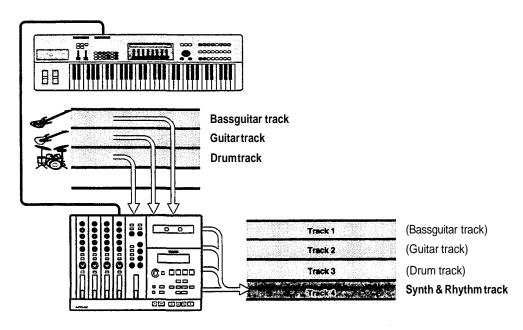
This technique is a combination of overdubbing (see "Overdub recording" on page 15) and ping-pong recording.
