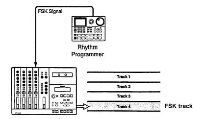
If your MIDI sequencer or rhythm machine is not equipped with a SYNC OUT connector, you may need a MIDI/FSK converter such as the Yamaha YMC10. You plug the MIDI/FSK converter in between your MIDI sequencer or rhythm machine and the MT4X to record FSK onto one of the tracks.
