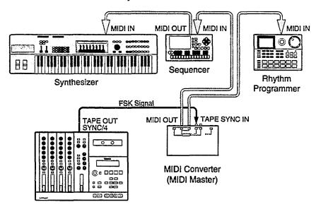
Some MIDI sequencers and rhythm machines can read FSK signals. You can plug this type of machine directly to the MT4X to synchronize to the recorded FSK signal.
