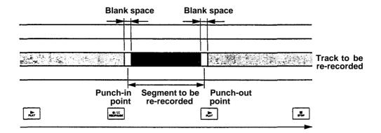
**Note:** When you perform a punch-in/out recording, you need to find a blank section of about 1 second for your punch-in and punch-out locations. This is because of the gap between the erase head and record/playback head. Otherwise you may find that you have accidentally erased material that was before or after the re-recorded segment.
