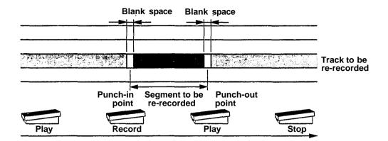
**Note:** When you perform a punch-in/out recording, you need to find a blank section of about 1 second for your punch-in and punch-out locations. This is because of the gap between the erase head and record/playback head. Otherwise you may find that you have accidentally erased material that was before or after the re-recorded segment.
