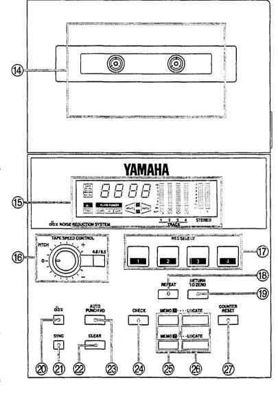
The tape speed (4.8/9.5) select key is used to switch the tape speed between 9.5 cm/sec and 4.8 cm/sec. 9.5 cm/sec will be selected automatically when the power is turned on.
