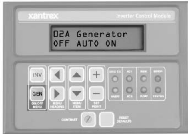
Figure 8-7 Generator ON/OFF Display
