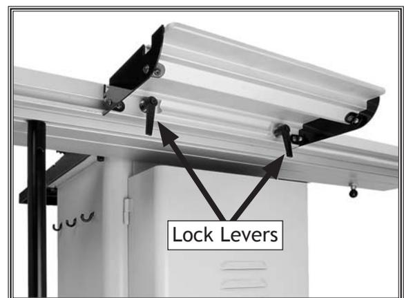
**Figure 17.** Locations of the extension table lock levers.
