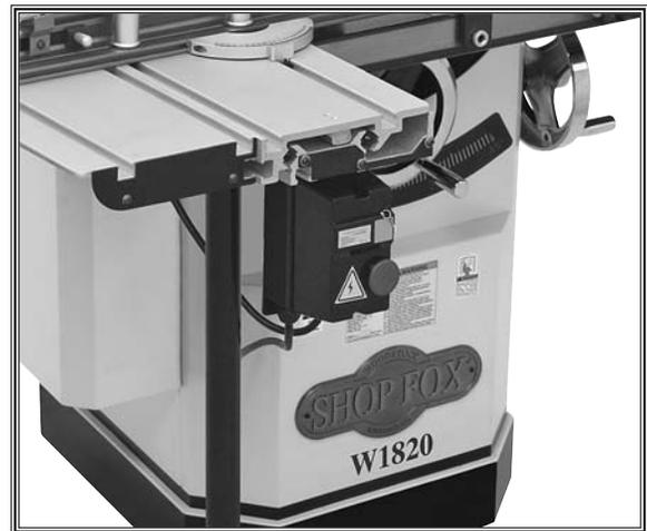
**Figure 4.** Example of relocating the power switch.
