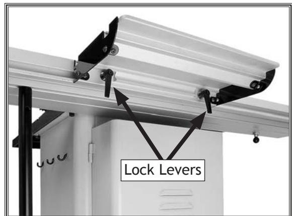
Figure 12. Locations of the extension table lock levers.
