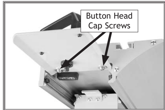
Figure 30. Sliding table handle attached to end of sliding table.
