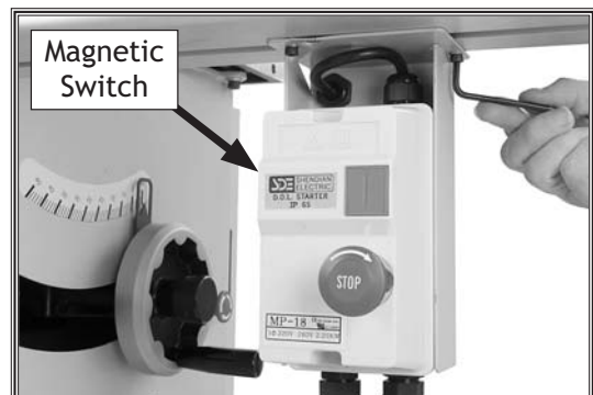
Figure 31. Magnetic switch installed.
