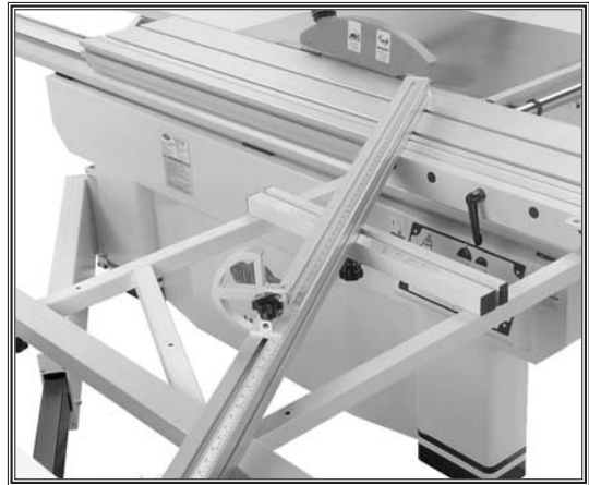
Figure 77. Fence set-up for 90° to 135° cuts.
