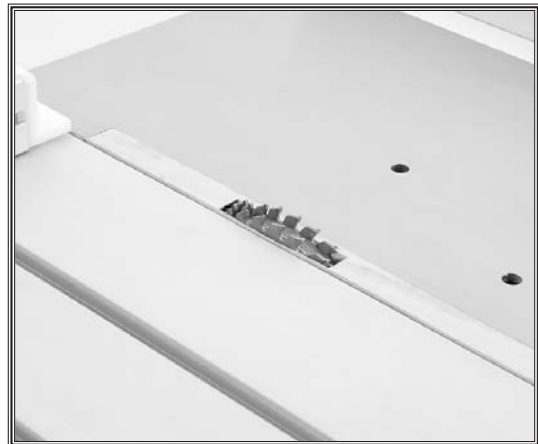
Figure 64. Dado blade raised into zero-clearance table insert.
