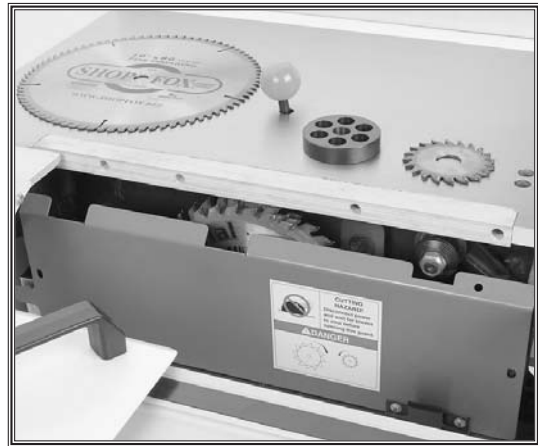
Figure 63. New zero clearance table insert installed.
