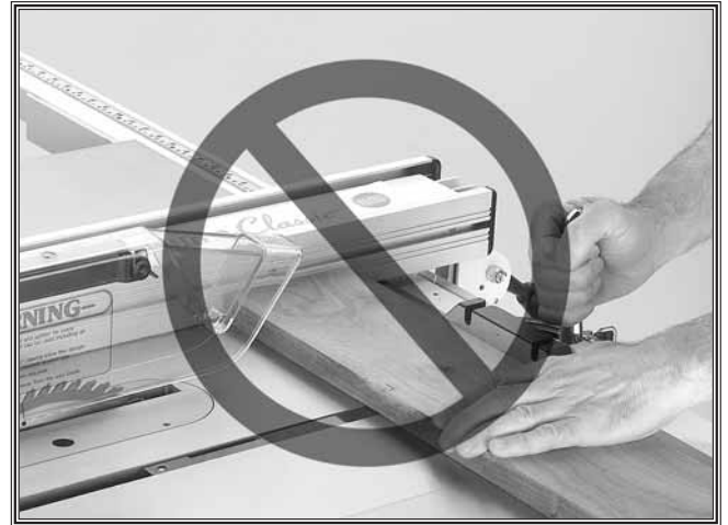
Figure 5. NEVER crosscut using the miter gauge with the fence.
