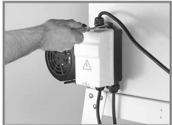
Figure 38. Installing magnetic switch.
