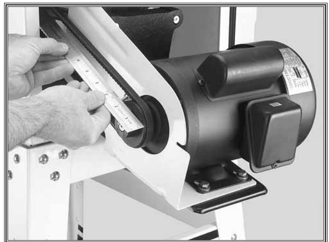
Figure 23. Checking pulley alignment with a straightedge.
