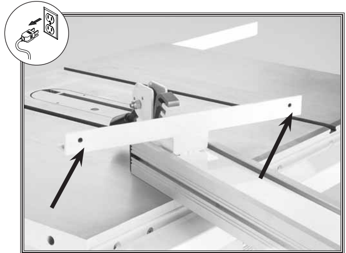
Figure 45. Fence adjustment setscrews.
