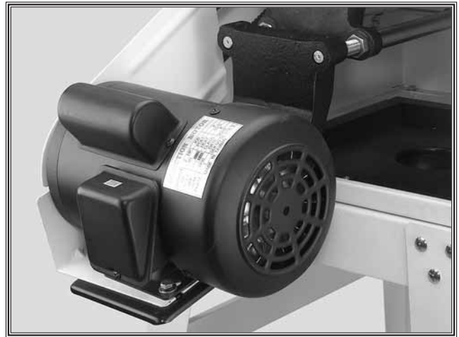
Figure 22. Motor installed on mounting bars.
