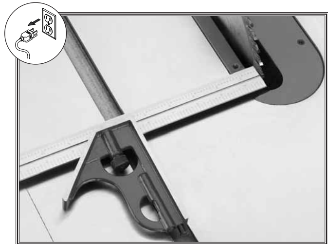
Figure 42. Checking blade/miter slot parallel.
