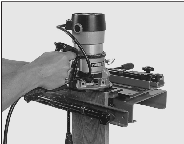
Figure 12 shows using the dovetail jig.
