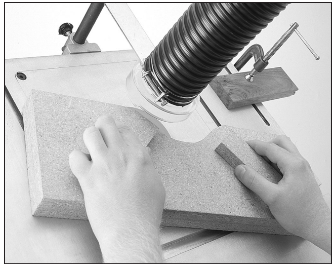
Figure 27. Work is supported by the guide bearing.
