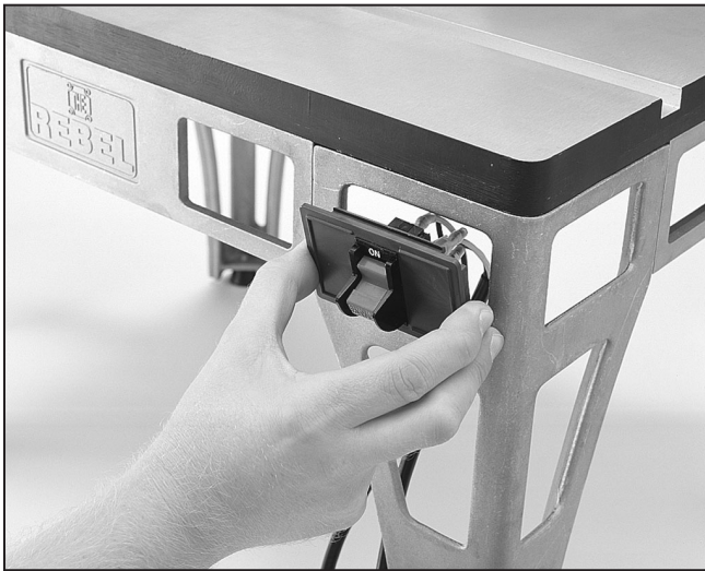
Figure 9. Installing the switch.
