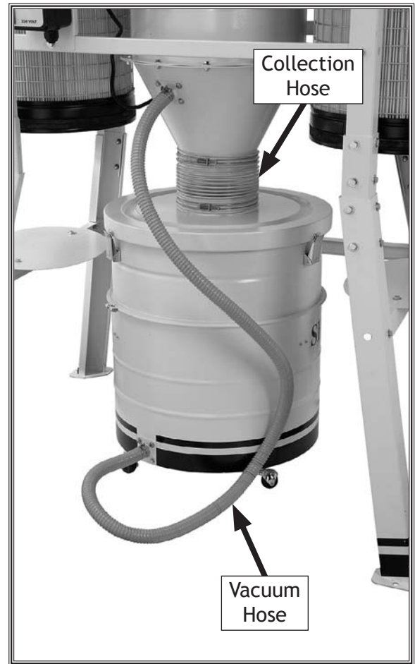
Figure 29. Collection and vacuum hoses installed.
