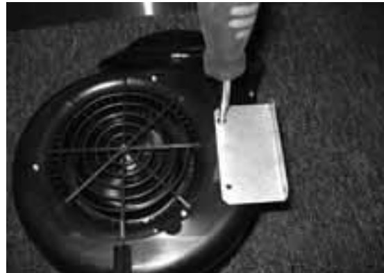
10. Attach blower brackets to blower using (2) screws on each side.
