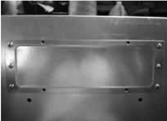
7. On the back of the hood, remove the (6) screws holding the rectangular cap.
