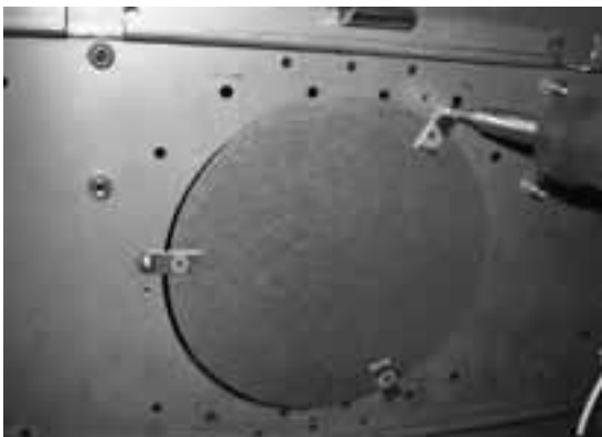
5. Cover blower opening on blower plate with 6" round metal cap. Attach with (3) screws provided.
