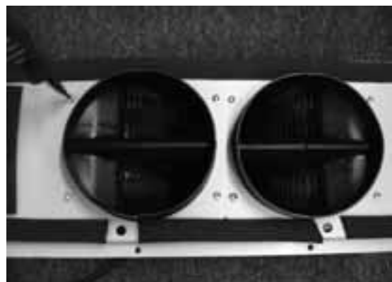
6. Use the blower removed from the single blower plate and install it into the dual blower plate.
