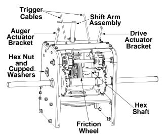
Figure 15 Viewed from the underside of snow thrower
