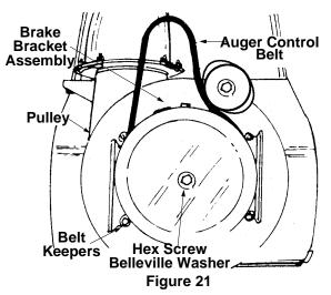
**Proper Adjustment** With the auger clutch lever in the disengaged position the top surface of the new belt should be even with the outside diameter of the pulley. To adjust, disconnect ferrule from the brake bracket assembly and thread ferrule in (towards idler) to increase tension on belt, out to decrease tension.
