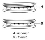
5. Turn on the burner. If the burner does not light, check cap alignment. If the burner still does not light, do not service the sealed burner yourself. Contact a trained repair specialist.
