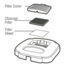
Diagram 5 Remove and replace charcoal filter To replace charcoal filter, push in release clip on filter cover. Lift charcoal filter out and discard. Wipe recess area clean with a damp soapy cloth, wipe clean and dry. Wash filter cover in hot soapy water, rinse and dry. Place new charcoal filter into recess with thin filter sheet down first. Replace filter cover and close to lock in place. See Diagram 5.
