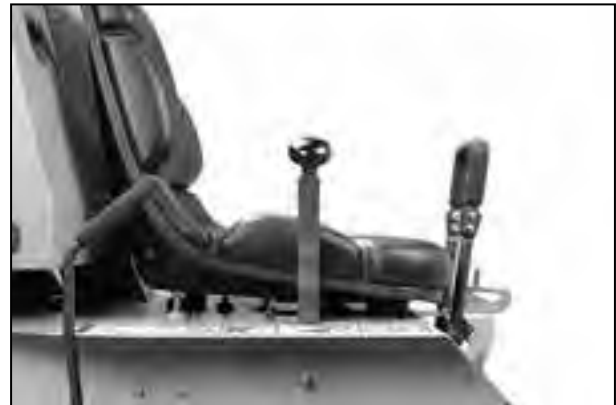
Correct FSC Lever NEUTRAL-PARK Position
