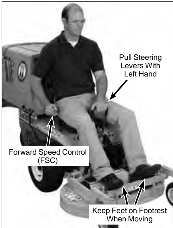
Correct Operator Hand Position on the Controls
