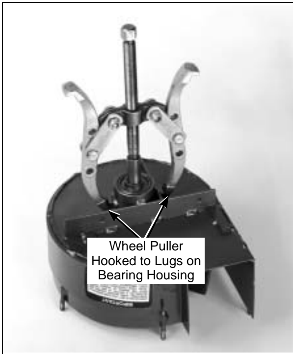
Pressing Blower Wheel Out of Housing
