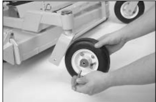
Deck Caster Wheel Installation
