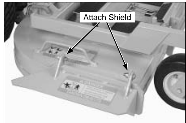
Deck Discharge Shield Installation
