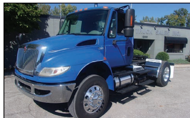
(2) 2011 & (2) 2012 INTL 4400 , MFD OR 9 270HP OR 210HP ALLISON AUTOMATIC TRANS, AIR RIDE SUSP, P/S, A/C, 158WB, 11X22.5, 100,000 THRU 145,000 MILES . . . . . 2011 $27,500 EA 2012 $28,500 EA
