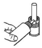
Failure to lubricate the piston properly with throat seal oil can cause premature wear and damage to piston and packings.
