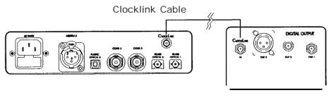
Wadia 27i Decoding Computer Clocklink-Equipped CD Transport
