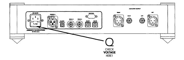
Check to make sure your *Wadia 27i Decoding Computer has* been manufactured for operation at your AC line voltage. Attempting to use your Wadia 27i Decoding Computer at any voltage other than specified on the rear of the unit may cause damage which is not covered by Wadia's warranty. If the voltage specified is different from your AC voltage, contact your Wadia dealer
