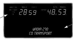
The bottom section is an alphanumeric display that shows the status of some of the Wadia 270 special functions.
