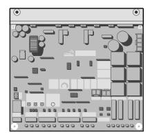
Using the connectors provided insert the wires from the motor units as shown in the diagram below. Insert the connectors in the proper receptacles on the Master/Slave Control Board. The 'Slave' gate opens first using the Overlap Delay (see page 28). If the gate opens in a clockwise direction, connect to the 'Outside' receptacle, if the gate opens in a counter-clockwise direction, connect to the 'Inside' receptacle
