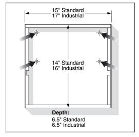
3. Position the control box and secure it to the mounting surface using the sealed washers provided (place the rubber side of the washers against the inside of the control box).
