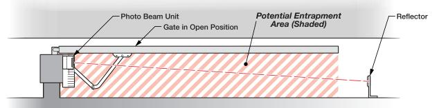
One or more non-contact sensors shall be located where the risk of entrapment or obstruction exists, such as the perimeter reachable by a moving gate or barrier.
