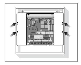
Position the control box in the desired place and mark the mounting holes.
