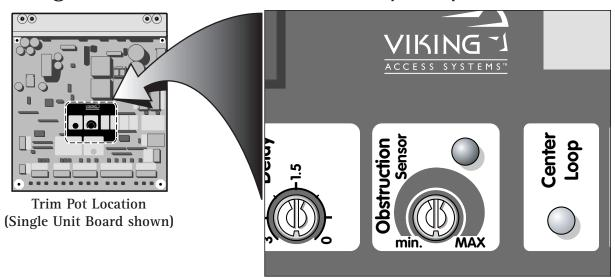
The Obstruction Sensor detects obstructions in the path of the traveling gate. The Trim Pot for the Obstruction Sensor adjusts the sensitivity level that triggers the Sensor.
