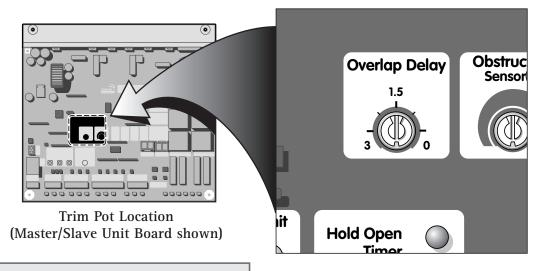
Setting the Overlap Delay Pot to any value other than zero will cause the master unit to delay in opening.
