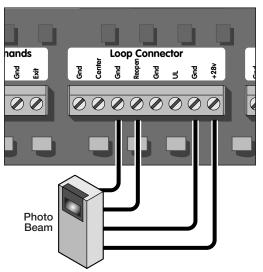
As an alternative to the Outside Reopen Loop, a photo beam unit can be used as shown.
