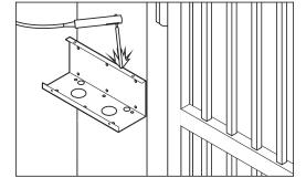
Note: Depending on type of anchor used, it may be required to enlarge the holes in the mounting chassis.
