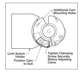
Note: Leave cover off until after the installation of the control box and the electrical installation. Verify that the operator opens and closes to the desired position under power. Make any adjustments as necessary.
