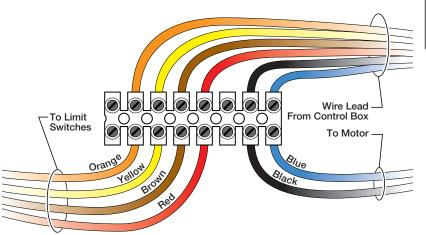
Note: Use this wiring diagram as a guide to connect the wires to the motor unit.
