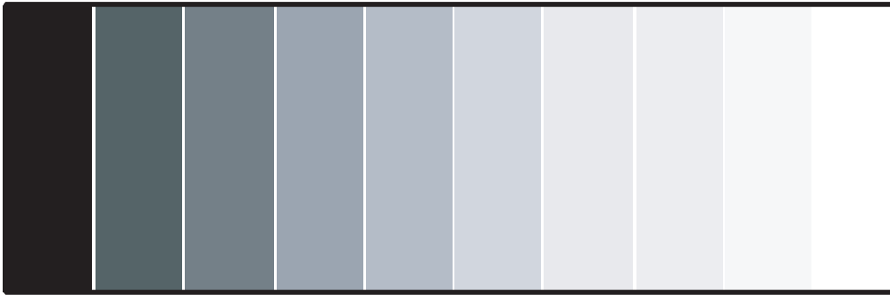
Figure 4-3. Typical Gray Bar Pattern for Adjusting Contrast
