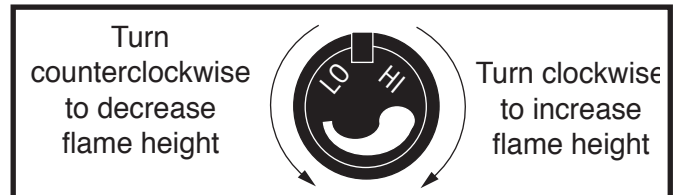
Fig. 25 Flame adjustment knob for Honeywell valve.
