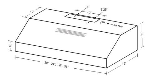
Note: Center of knockout is 8.25" from center of hood & 2.5" from back.
