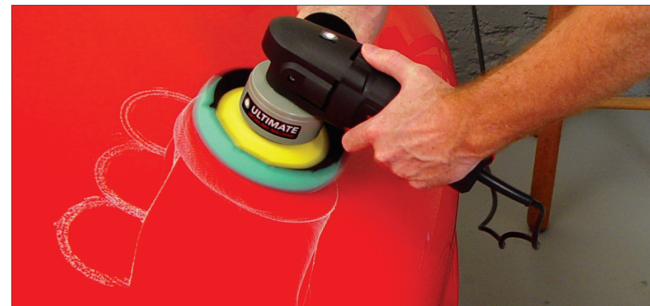
Step 4: Start polisher at low speed. Start the polisher at a low speed (2 on the dial), making sure to press the pad against the car before switching the machine on. Allow the polish to load into the pad and distribute over the surface area before increasing speed.
