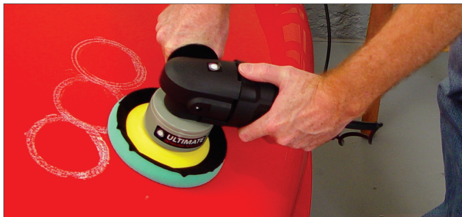
Step 3: Distribute polish over the work area. Distribute the polish over the work area. If you don't, the polish will sling off of the pad. You can dab it, as I have done here, or smear it.
