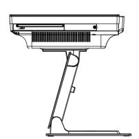
For viewing clarity, you can tilt the desktop LCD from 30 to 75 degrees from vertical.
