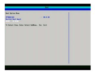
Using the Arrow **UP** or **DOWN** key(s) on the keyboard to select the CD/ DVD drive you are using. When selected press **ENTER**.
