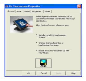
Click on the Align button. This launches the align/calibration program. A window similar to the one shown below will open. Follow the instructions to align/calibrate the touchscreen.
