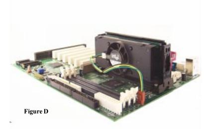
Figure D above shows a properly installed SECC2 CPU using the retention module. Note the direction of the CPU fan and the way in which the cable is connected.
