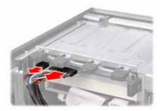
3. Unfasten the LED module and slide it out as shown to lift it free of the chassis.
