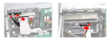
3. Unfasten the installed drives or the empty drive brackets from the chassis in the direction of the arrow shown.
