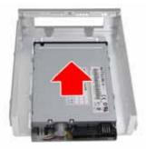
9. Secure the FDD in place using four screws.
