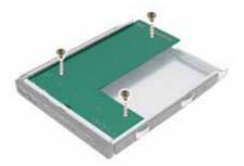
5. Slide the LED control board from the bracket as shown.
