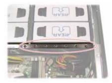
2. Secure the supplied long card holder to the fan cradle with one screw.
