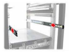
9. Lift the unit and then insert the inner slide rails into the middle rails.
