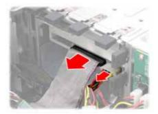
3. Unfasten the DVD-ROM drive and slide it out of the chassis in the direction of the arrow shown.
