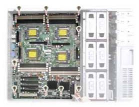
3. Carefully lift the motherboard from the chassis.
