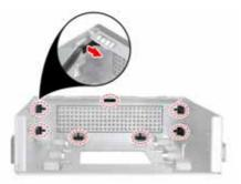
6. Remove the front panel and the inner piece as shown.
