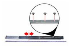
6. Install the two small brackets (A) to each mounting bracket (front x 2, rear x 2) in the rack.
