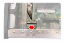
2. Secure the security tab with two screws.
