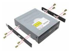
5. After replacement, insert the unit to the chassis following the above steps in reverse.
