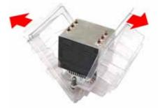
9. Place the fan and heatsink on top of the CPU and attach with two screws as shown.
