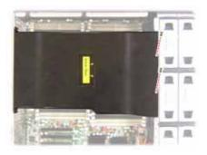
2. Remove the air duct and locate the memory slots on the motherboard.
