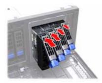
13. The expansion HDD numbering is indicated as below. Right to left: HDD9, HDD10, HDD11, HDD12
