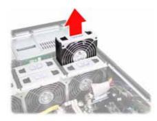
2. Replace a new fan into the fan cradle following the above steps in reverse.
