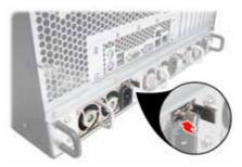
2. Press the latch and the handle together as shown.
