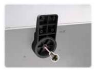
case. When fitted, each foot should rotate about 90°.
