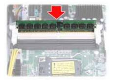
When inserted properly, the memory slot locking levers lock automatically onto the indentations at the ends of the module.
