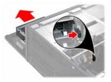
3. Remove the two rails from the drive bracket.
