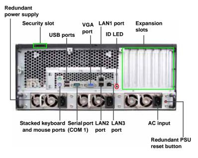
**NOTE**: The buzzer sounds during power failure or abnormal condition. Press the Redundant PSU reset button to return the power supply units to their default states.
