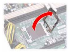
6. Place the CPU in the socket as shown, making sure that pin 1 is located correctly.
