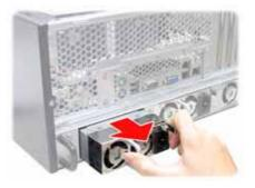
4. Place the unit with the new power supply unit and secure by tightening the thumb screw.
