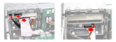
2. Unfasten the installed drives or the empty drive brackets from the chassis in the direction of the arrow shown.
