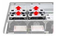
2. Unfasten an empty drive bracket from the chassis in the direction of the arrow shown.
