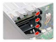
3. Slide all the drives or the brackets out of the chassis.
