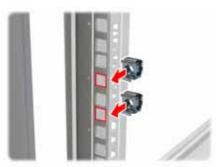
Secure the outer rails to the rack using four M6 screws (B) for each side. Secure the mounting brackets from outside, not inside, of the rack.
