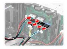
15. Connect the other end of the SATA/SAS cables to the connectors on the PCI-E RAID card.
