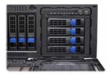
Connect the power and data cables to the SATA/SAS backplane. SATA/SAS connectors on the M1216-P backplane are indicated as below. Top to bottom: J1, J3, J5, J7
