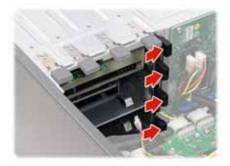
4. Slide all the drives or the brackets out of the chassis.
