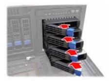
7. The expansion HDD numbering is indicated as below. Top to bottom: HDD9, HDD10, HDD11, HDD12
