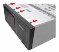
2. Remove the door assembly from the four holes located on the lower edge of the server.
