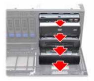
5. Slide all the drives or the brackets back into the chassis vertically.
