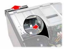
5. Use a thin tool such as a flat screwdriver to pry open the front panel of the drive bracket as indicated.
