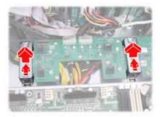
4. Remove the ten screws securing the fan board to the chassis.
