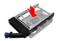
4. Secure the hard drive in place using four HDD screws.
