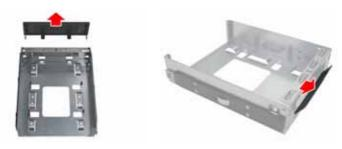
7. Install the FDD front panel to the front of the bracket.
