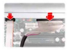
5. Place the SMDC card in the PCI slot as shown.
