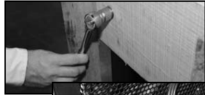
Some units have a polyester strap that secures the cabinet to the shipping skid. Cut this polyester strap and remove the wood skid.
