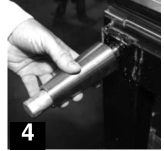
4 Thread leg into cabinet bottom frame rail.
