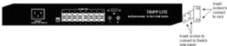
Figure 7 Connecting the L-shaped bracket
