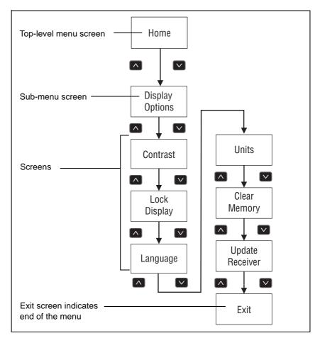
Figure 4.4 shows the structure of a typical sub-menu, such as *Display Options*.
