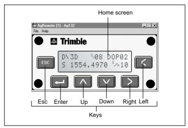
Figure 4.3 AgRemote window and navigation keys.
