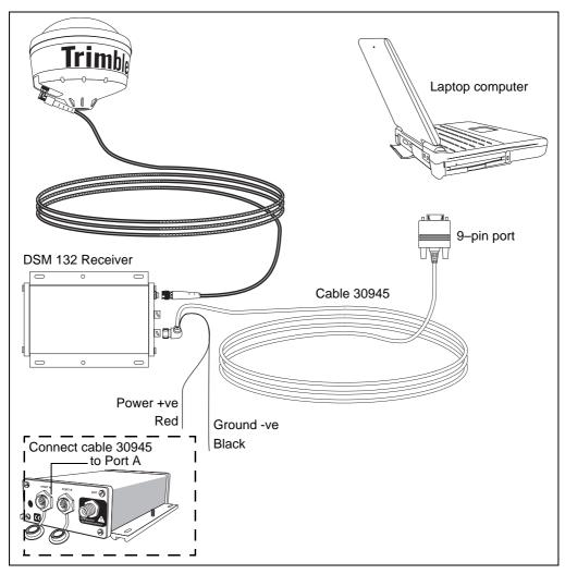
Figure 4.2 Connecting the receiver to an office computer
