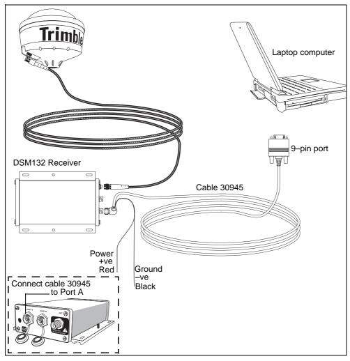
Figure 3.4 Connecting the receiver to a laptop computer
