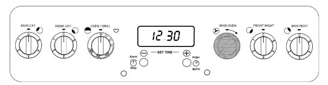
• Turn the main fan oven temperature control to the required setting.
