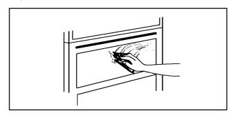
DO NOT ATTEMPT TO REMOVE ANY OF THE CONTROL KNOBS FROM THE APPLIANCE AS THIS MAY CAUSE DAMAGE AND IS A SAFETY HAZARD.
