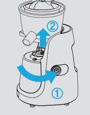
Disassemble Vertical Auger, Juicing Screen and Pulp Wiping Assembly.
