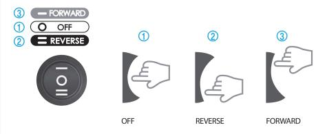
\*While operating 'FORWARD' switch, please press 'OFF' switch and wait until the appliance stops completely before using the 'REVERSE' switch.
