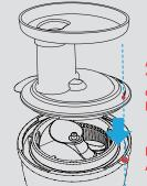
Align mark at "OPEN" position on the Auger Housing Lid
