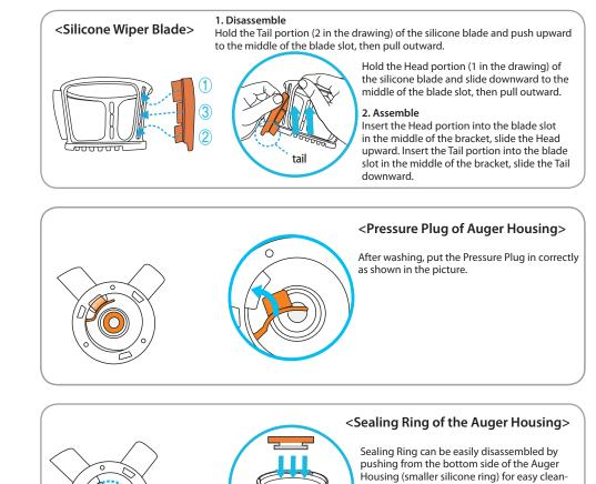
Housing (smaller silicone ring) for easy cleaning. After it is thoroughly dried, put the sealing ring properly back in its place. Push the sealing ring (with the larger side facing up) back in place from the inside of the Auger Housing.
