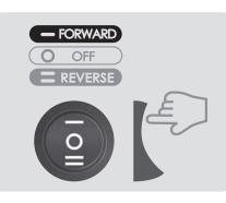
After juicing and self cleaning, turn off the machine. The Feeding Chute Assembly may not open well if the extraction is not finished. If this is the case, please see page 12 on "how to disassemble.
