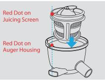
Connect the Feeding Chute Assembly to the Auger Housing. Align the mark of the "OPEN" position on the Auger Housing Lid to the red dot on the Auger housing.
