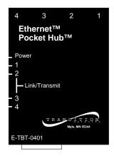
When centrally located in a small installation, the 0401 Pocket Hub can be used to connect up to four terminal devices to a
