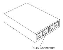
Four (4) 10BaseT RJ-45 jack connectors are located at one end of the 0401 Pocket Hub. The RJ-45 jacks support connection to shielded or unshielded 100 ohm twisted pair 10BaseT cable.
