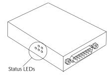
Power and Link/Transmit status LEDs are located at the side of the 0401 Pocket Hub. The **Power** LED indicates connection to power. The **Link/ Transmit** LEDs track the four 0401 Pocket Hub connections to 10 BaseT.
