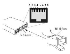
The two active pairs in a 10BaseT network are pins 1 & 2 and pins 3 & 6. Use only dedicated wire pairs (such as blue/white & white/blue, orange/white & white/orange) for the active pins.
