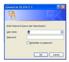
Leave the User name field blank and enter read write or read only Password. Press OK. Default password is trango. After logging on, the system information screen will be displayed.
