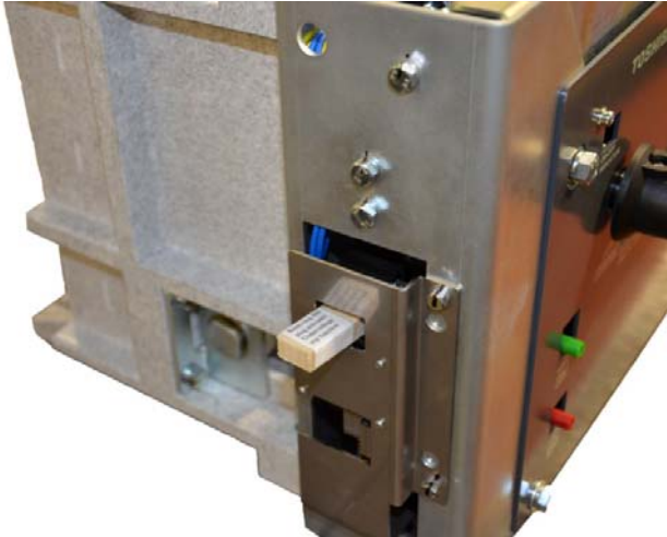
Figure 30 Plug Installed in UV Trip Device
