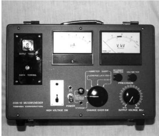
Figure 32 Toshiba Portable Vacuum Checker
