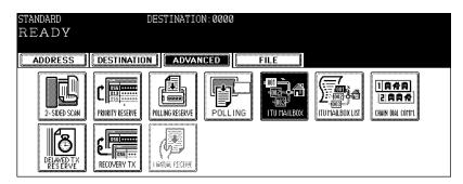
**3** Press the [CONFIDENTIAL] (or [BULLETIN BD.] or [RELAY]) button, and then press the [BOX DELETE] button.
