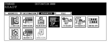
**3** Key in the password (4 digits) if the password check is set for the remote Fax, and then press the [ENTER] button.
