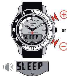
b) + / - : stop the count, the watch does not switch to standby mode
