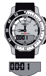
Dive mode active - elapsed time in LCD, minutes hand shows depth in meters or feet on bezel, hours hand shows dive speed in m/min or ft/min on dial
