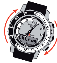
Turn the watch more than a complete revolution on a horizontal surface (e.g. a table) in an environment free from magnetic interference, at a rotation speed of around 30° per second. Total time: 20 seconds maximum
