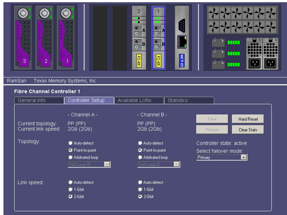
Figure 7-1: Controller Setup via Web Interface
