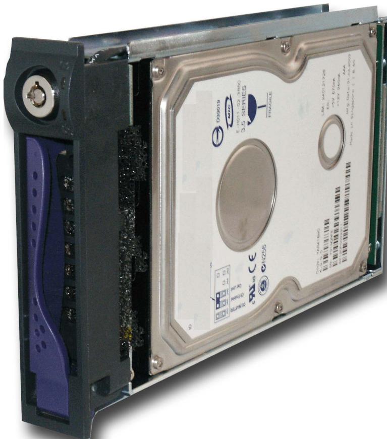
Figure A-6 120 Gigabyte Replacement Hard Drive
