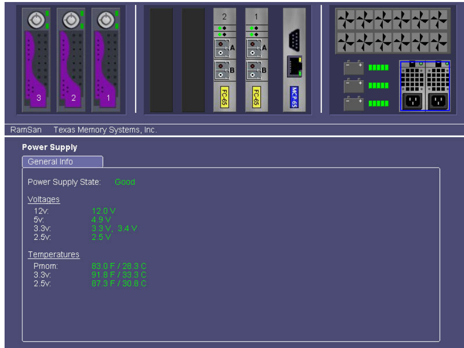
Figure 5-7: Power Supply Status via Web Interface
