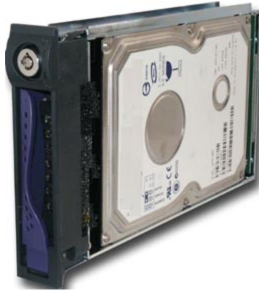
Figure A-6 120 Gigabyte Replacement Hard Drive
