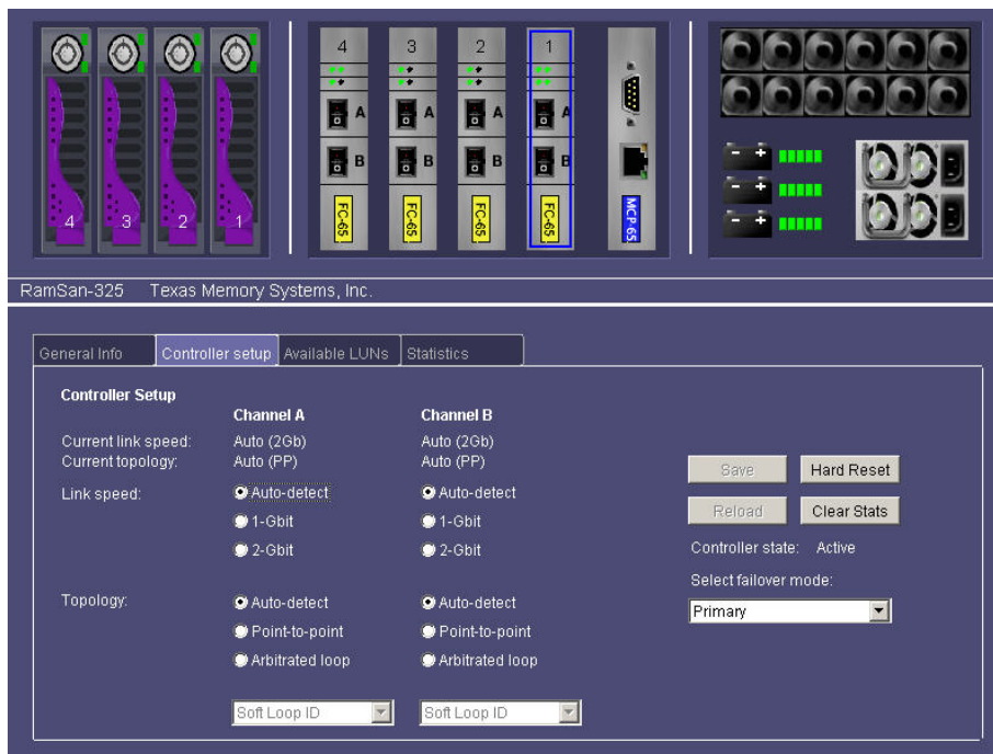
Figure 7-1: Controller Setup via Web Interface
