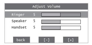
Press  $\Delta$  or  $\nabla$  to choose which level you want to adjust. Pressing [-] will decrease, while pressing [+] will increase the volume level for the item displayed. The change will take place immediately. Pressing the soft key button under the word **back** or the **Select** button will return you to the main screen. The following volume levels can each be individually adjusted:
