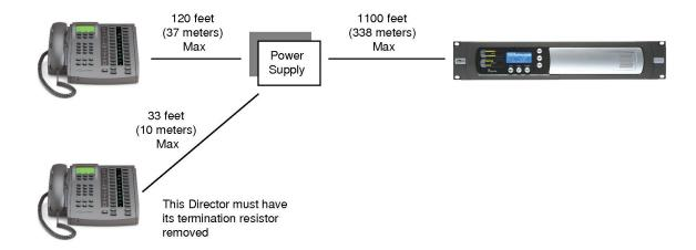
To connect two Desktop Directors to one port, a power supply and RJ-45 modular splitter is required.
