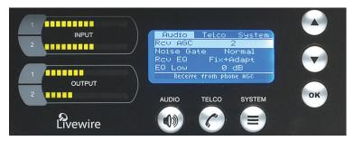
Pressing any menu button (Audio, Telco, or System) twice displays the Status screen.
