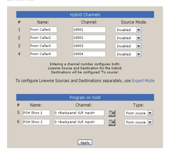
There are 4 hybrid channels. You can enter the Livewire text name and channel number or accept the defaults. Livewire channels are two-way, so this applies to both the send and receive audio. A Livewire enabled mixing console such as the Axia Element, when taking one of these as a source, will automatically connect both directions and provide the mix-minus. Cool, eh?
