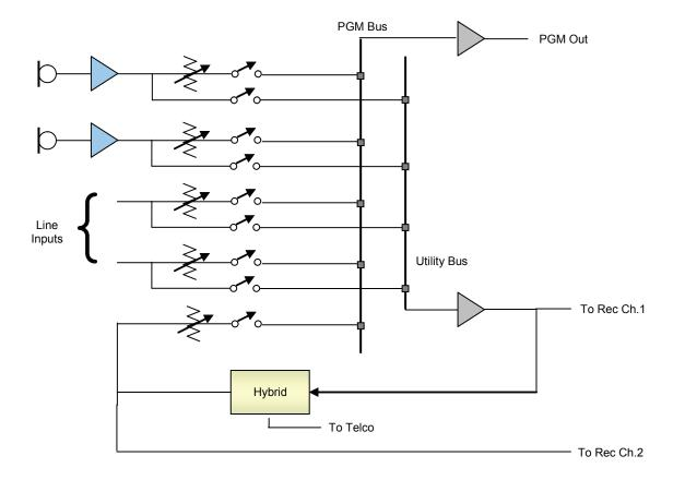
The Nx12 has multiple hybrids and works best if two faders can be assigned to the telephone system with two associated mix-minuses, one for each telephone line column on the Director. This is probably not going to be easy with an older console. But the Nx12 has an option to work with a single external mix-minus by making an internal cross-connection of the hybrids. See Section 5.7 for more on this.
