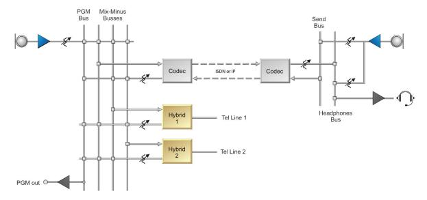
A problem could result from a hybrid with too much leakage and the codec delay. If the hybrid isn't doing a good job of preventing the send audio from leaking to its output, the remote mixminus is corrupted. Remember, if any of the announcer audio from the remote site is returned, it will be delayed by the digital link, causing an echo effect in the announcer's headphones.
