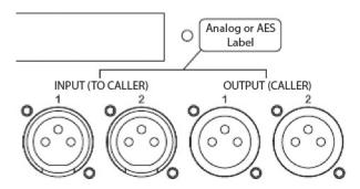
have the shield wire connected only on one end to prevent ground loops. Older equipment with a transformer output stage may need a terminating resistor across pins 2 and 3; consult the manual for your equipment for how to use it with high impedance inputs.
