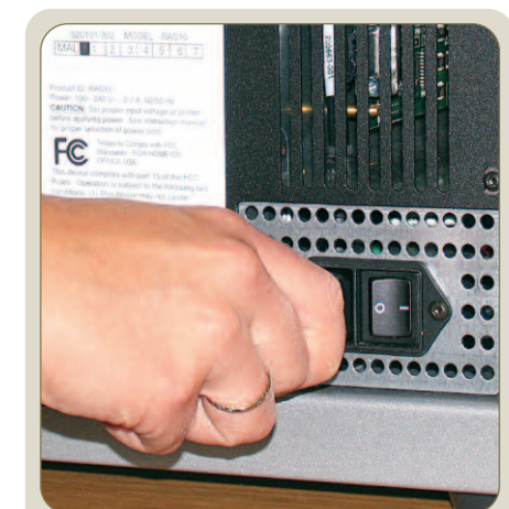
3 Insert the Power cable
