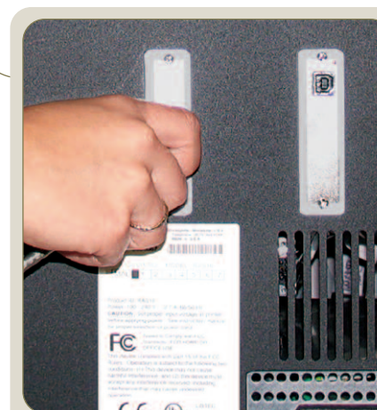
1 Insert the FireWire® cable
