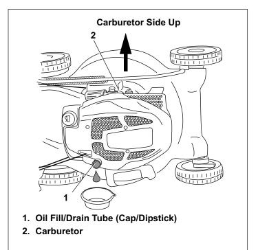
Figure 33. Draining Oil Sump
