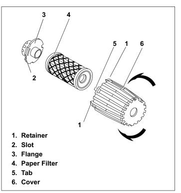
Figure 50. Air Cleaner Type "C" Assembly
