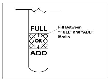
Figure 6. Engine Oil Level
