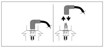
Figure 2. Disconnecting/Connecting Spark Plug
