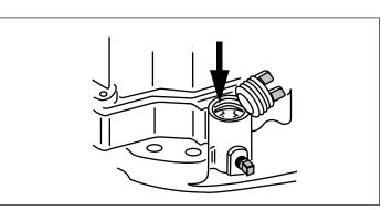
Figure 9. Engine With Oil Fill Plug
