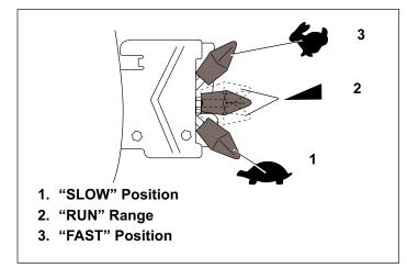
Figure 19. Start/Choke Control Positions
