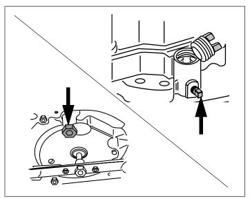
Figure 41. Oil Drain Plug Locations
