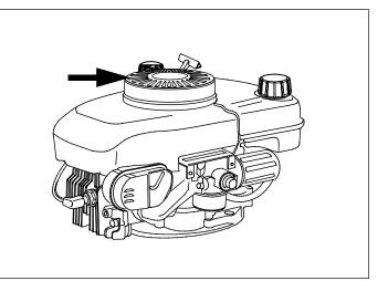
Figure 1. Typical Flywheel Guard Location
