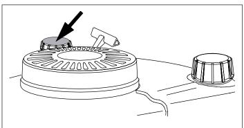
Figure 8. Oil Fill Cap Dipstick
