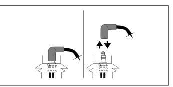
Figure 28. Disconnecting/Connecting Spark Plug
