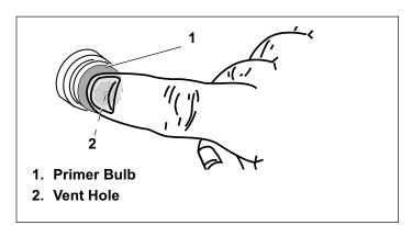
Figure 20. Pressing Primer Bulb
