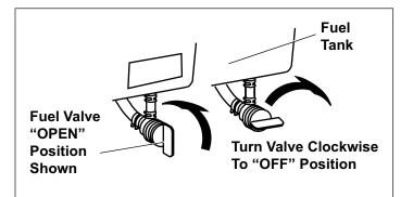
Figure 11. Fuel Valve Positions
