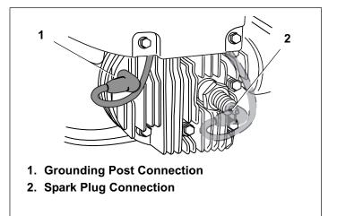
Figure 36. Typical Grounding Post/Spark Plug Connection
