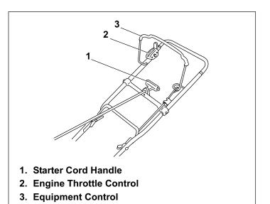
Figure 25. Typical Engine Controls
