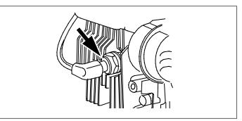
Figure 37. Typical Spark Plug Connection
