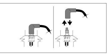
Figure 53. Disconnecting/Connecting Spark Plug
