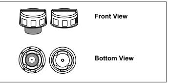
Figure 10. Possible Anti-Splash Fuel Fill Cap(s)
