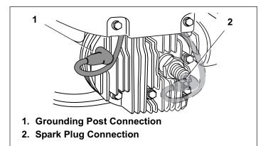
Figure 3. Typical Grounding Post/Spark Plug Connection
