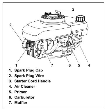
Figure 15. Engine Components
