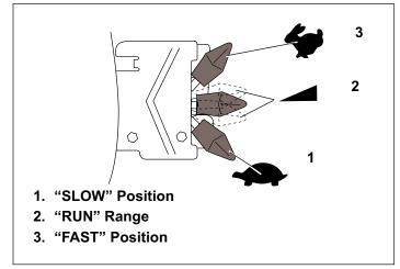
Figure 23. Start/Choke Control Positions
