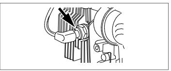
Figure 45. Typical Spark Plug Connection
