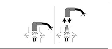
Figure 35. Disconnecting/Connecting Spark Plug
