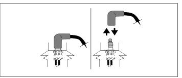
Figure 43. Disconnecting/Connecting Spark Plug
