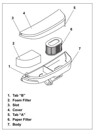
Figure 51. Air Cleaner Type "D" Assembly
