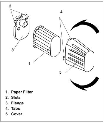
Figure 52. Air Cleaner Type "E" Assembly
